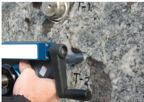
Figure 12.7 — Portable tensile pull testing equipment is attached to the metal disc. Test equipments exerts a “pulling” force on the disc and cored stone section (to the point of failure) to measure its tensile bond strength.
