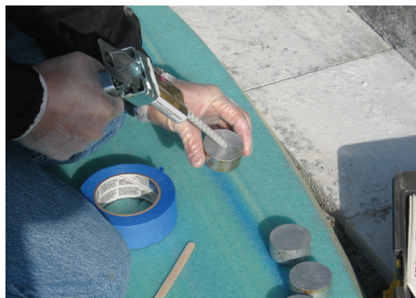
Figure 12.5 — 2" (50 mm) diameter metal disc to be adhered to the stone surface with a two component epoxy resin adhesive.
