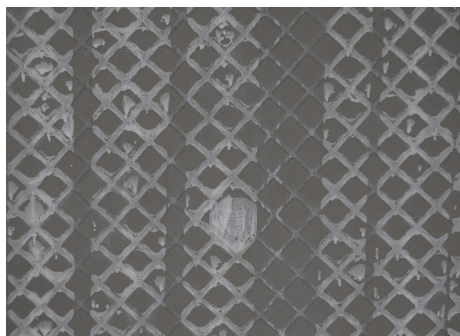
Figure 10.3 — Example of kiln release present on tile back.
