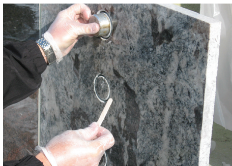
Figure 12.6 — Metal disc adhered to the stone surface with a two component epoxy resin adhesive.
